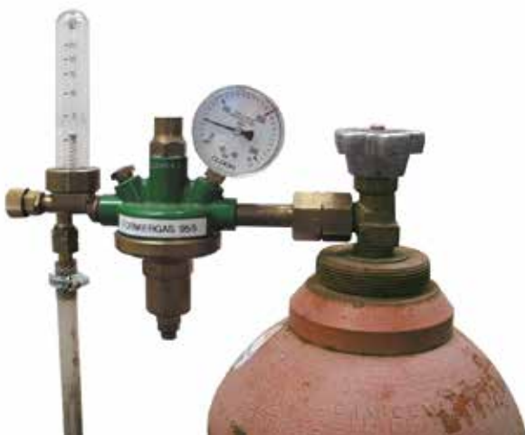
Pressure reducing valve with assembled flow meter
