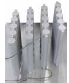
Titanium rods after heat treatment in NR 50/11 in argon atmosphere
