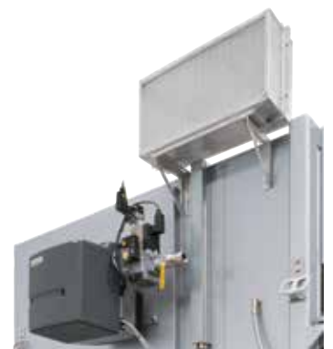
Direct gas-firing at a chamber dryer
