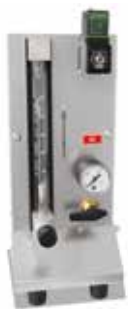
Gas supply system for non-flammable protective or reactive gas with shutoff valve and flow meter with regulator valve, optionally with magnetic valve
