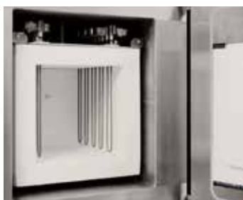
Molybdenumdisilicide heater and fiber insulation
