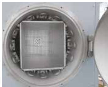
Inside heating in retort furnaces NRA ../06
