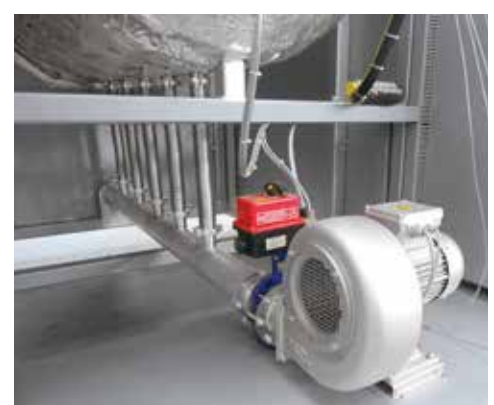
Fan cooling, hot-wall retort furnace NRA 400/03
