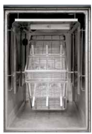
Motorized rotary rack with baskets for moving the charge during heat treatment
