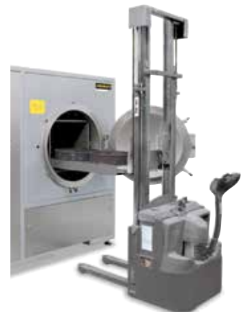
Charging of the retort furnace NRA 300/06 with a pallet truck
