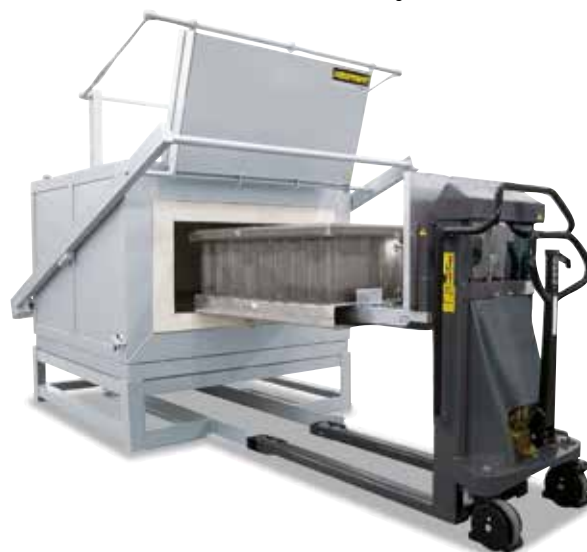
Guiding track at the base frame
