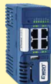
Router for remote maintenance
