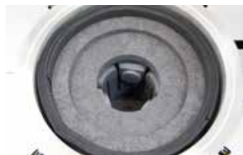
Graphite heating module
