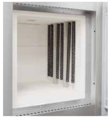
Vertically mounted SiC rods and optional perforated air inlet tubes of the debinding system
