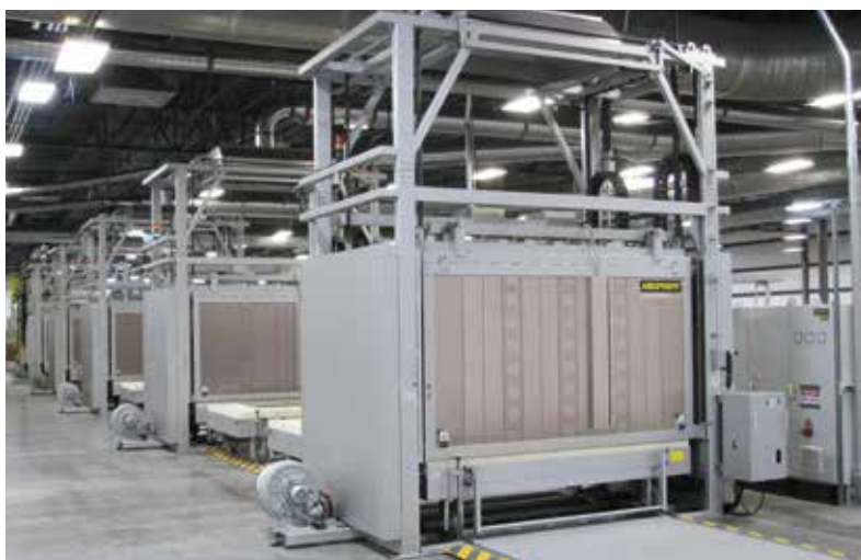
Lift-top furnace H 3630/LT DB200 for debinding and sintering
