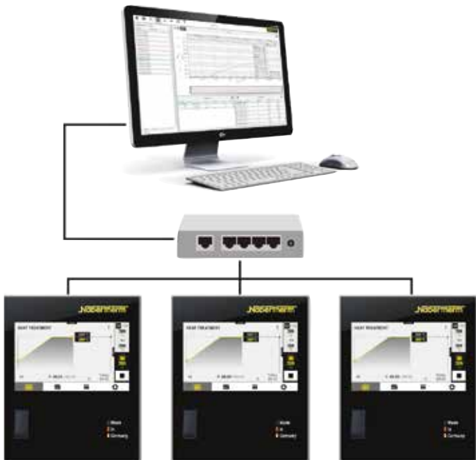
Example lay-out with 3 furnaces
