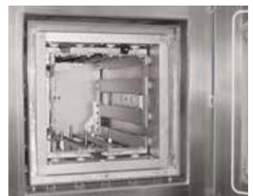
Tungsten heating chamber
