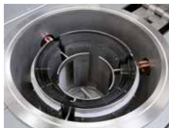
Cylindrical retort with tungsten heating
