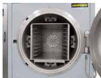
Retort with internal heating and process chamber
