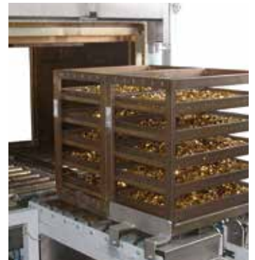
Continuous furnace for bulk materials in baskets
