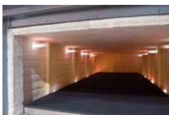
Furnace chamber with eight high-speed burners
