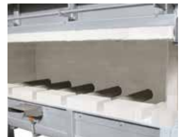
Indirect gas firing with radiation tubes
