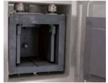
Graphite heating chamber
