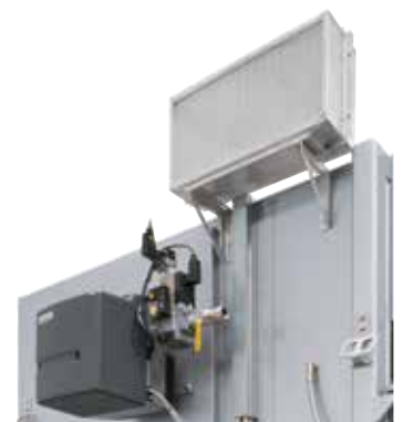
Direct gas-firing at a chamber dryer
