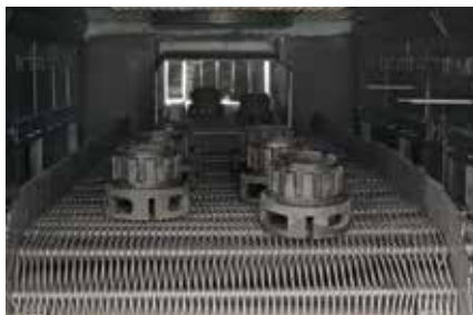
Mesh belt drive in a continuous furnace
