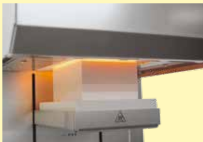
Automated table lowering for fast cooling
