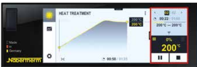
Detailed overview of process information including setpoint, actual value and switched functions
