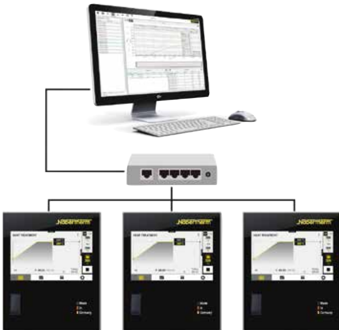
Example lay-out with 3 furnaces
