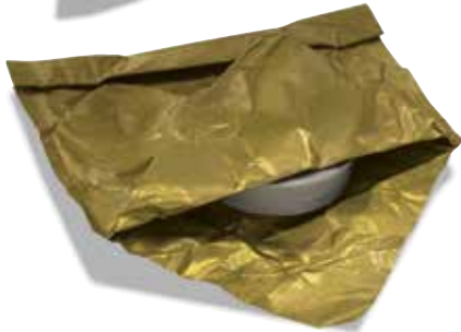
Workpieces in foil heat treating
