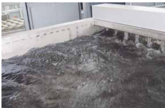
Powerful circulation of quenching medium
