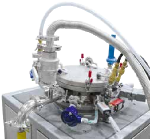
Retort with vacuum and protective gas line, cooling water connections as well as thermocouples and pressure sensors
