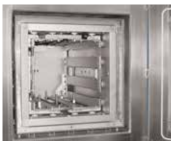
Molybdenum or tungsten heating chamber
