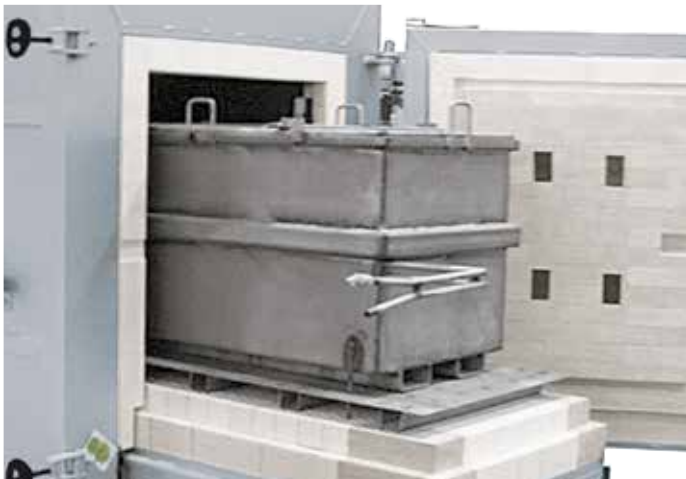
Protective gas box used in a large bogie hearth furnace with air circulation
