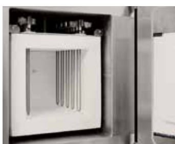
Molybdenumdisilicide heater and fiber insulation
