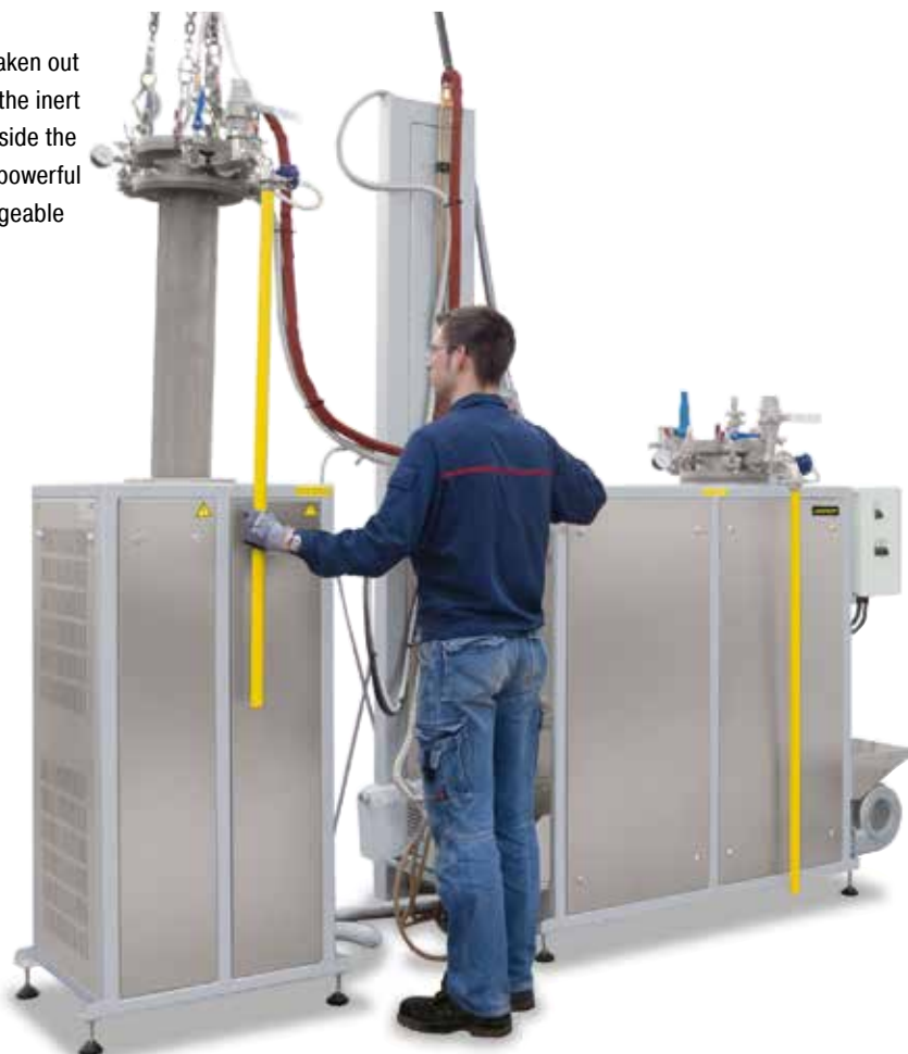
Retort furnace SR 170/1000/11 with changeable retort and cooling station
