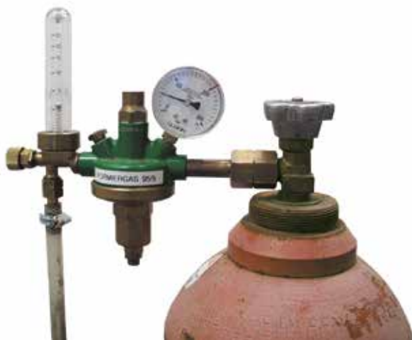
Pressure reducing valve with assembled flow meter
