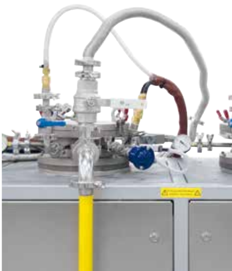
Exchangeable retorts with supply and measuring lines
