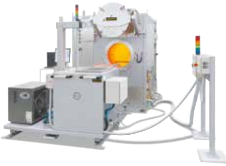
Hot-wall retort furnace NR 50/11 with semi-automatic quenching device for hardening of steel or titanium
