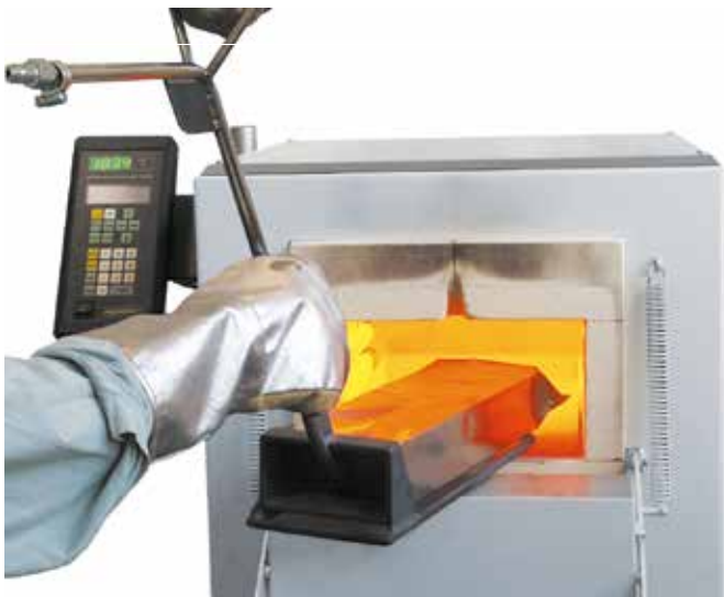
Hardening in annealing tray with alloy bag
