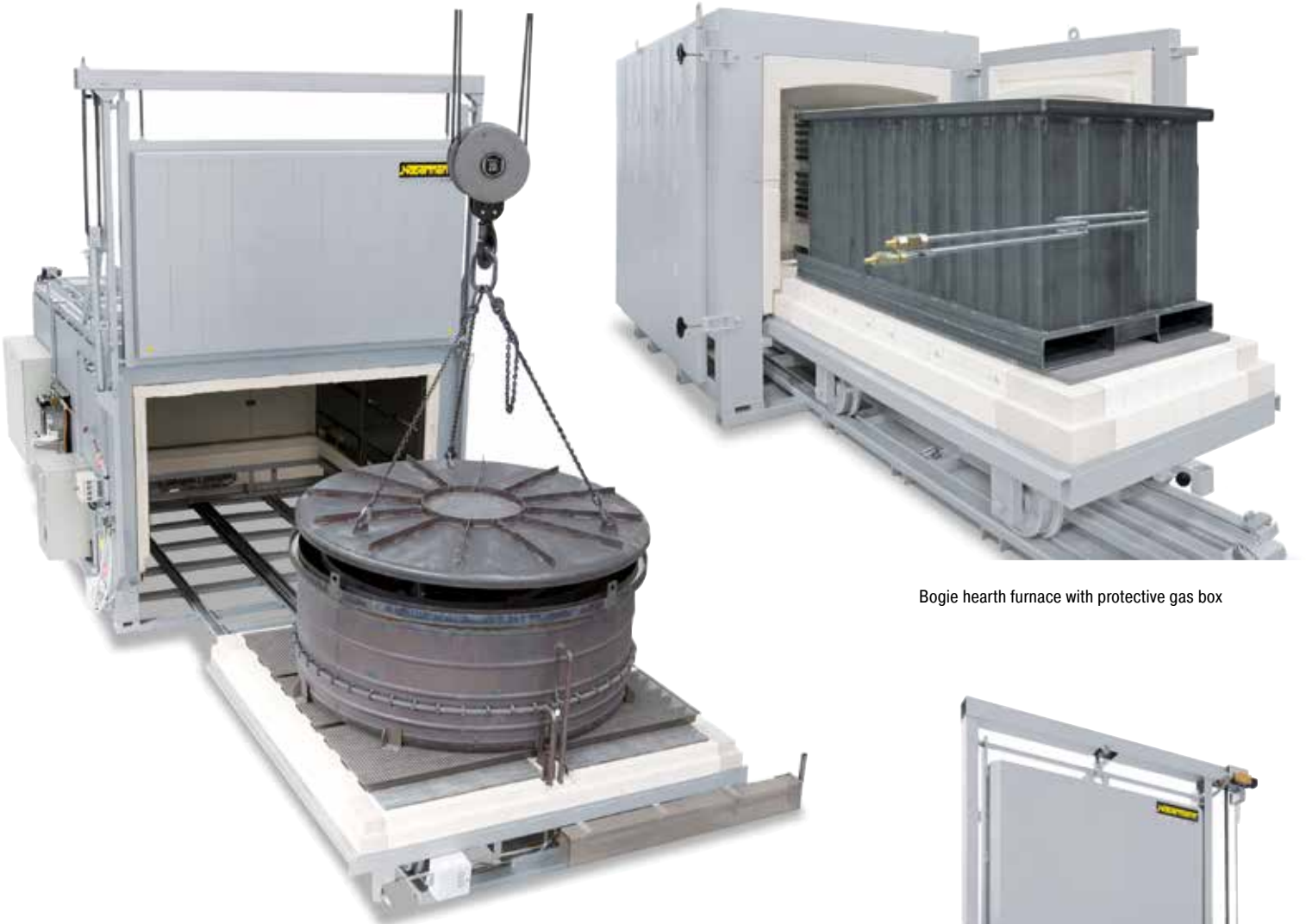
Forced convection bogie hearth furnace W 5290/85 AS with annealing box for heat treatment of coils under protective gas
