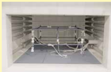
Measurement set-up in an annealing furnace
